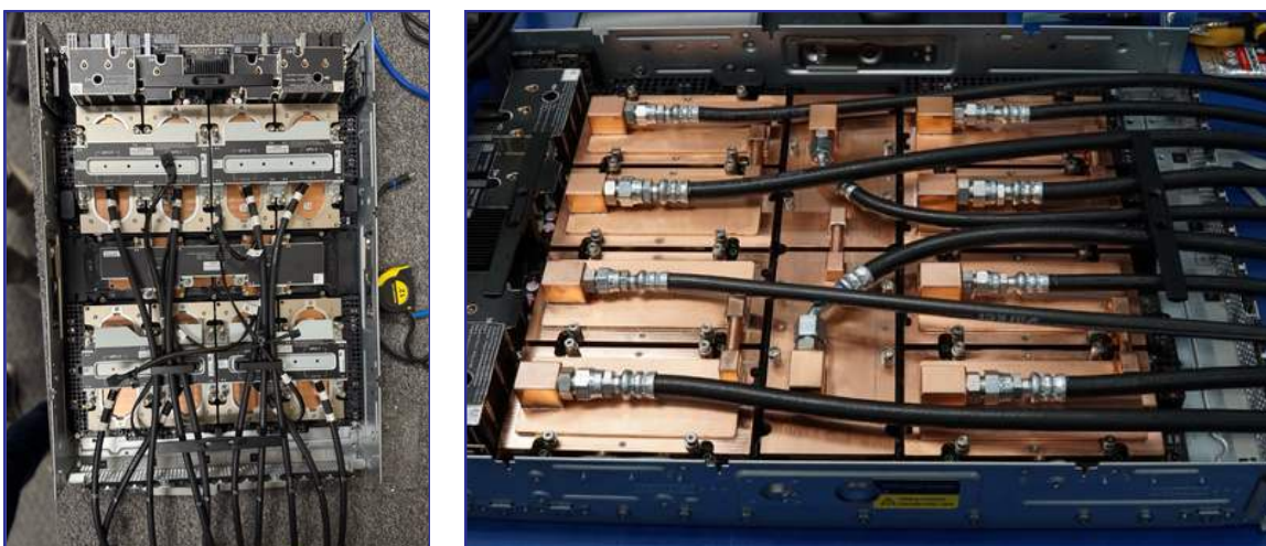
Figure 1. Before and after. Left: the tested Dell PowerEdge XE9680L GPU tray with its factory-installed single-phase cold plates. Right: the same server retrofitted with Accelsius NeuCool two-phase cold plates. All other server hardware was unchanged.
