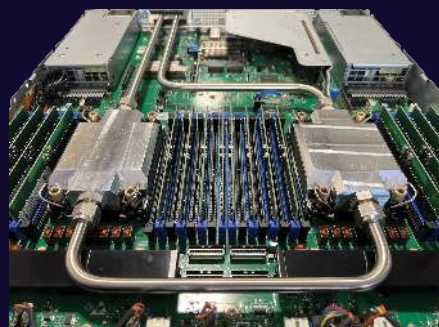
2 Socket CPU server showing Vaporators and metal internal tubing
