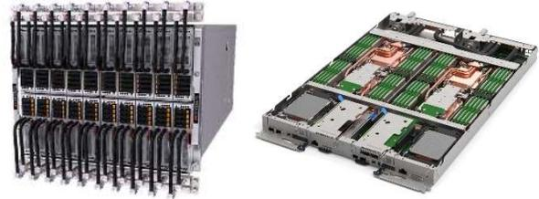
Fig. 1 (Left) Supermicro SuperBlade [8] with servers and cold plates in vertical orientation. (Right) Lenovo ThinkSystem SD650 V3 Neptune DWC Server [9] with horizontal upward cold plates.
