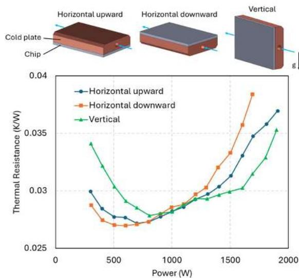
Fig. 2 Thermal resistance of a cold plate under different orientation conditions.
